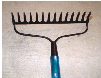
Figure 3: Rake head used to recover submerged vegetation attached to a 16-foot pole.
